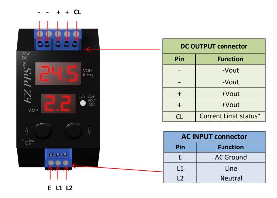
\*CL Output: Current-within-Limit output is a PNP transistor output capable of sourcing 100 mA at 24 VDC. The output is ON (24VDC nominal) when output current is less than programmed limit, the output is off otherwise.
