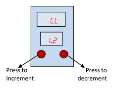
Press both buttons together to save the changes. The unit returns to its normal display after saving the new current limit.
